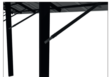
Linking of the diagonal to the C-post
