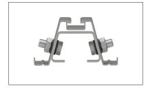
Bild 6.3 - 3 Installed Connector with Module support rail
