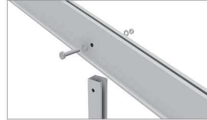
Connection detail leg - rafter
